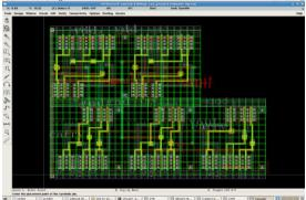
Fig.4.5. Layout of full adder.
