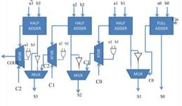
Fig.2.2. Proposed CSLA using CBL.
