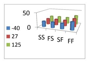
Fig.4.10. Variation of power with temperature and process corner.
